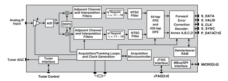
The Broadcom BCM3510 is a VSB/QAM digital receiver, compatible with both North American digital cable television and digital terrestrial broadcast television standards. The BCM3510 is capable of receiving all Standard-Definition and High-Definition digital television formats (SDTV/HDTV).
